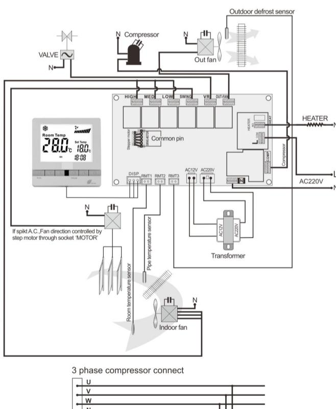
the SWING-MOTOR plug. The output plug for stepping motor is 6-pin plug, with two sides as common port (12V). In installation process, the common port of swing motor plug must be inserted into one common port of stepping motor's output plug. If stepping motor works in the wrong direction, change the common port of the swing motor into the other common port of the output plug of the stepping motor.
