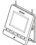
Step 7: Hang above two hooks in angle of 30 degrees, must put in place.
