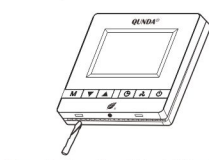
Step 2: Pry it a little bit to disassemble the thermostat.
